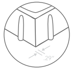
Spacers protrude 0.29” (7.5 mm) from the main body.
